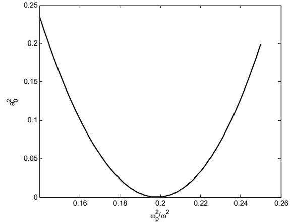
**Fig. 1.** Variation of normalized whistler amplitude  $a_0^2$  with  $\omega_p^2 / \omega^2$  for  $\omega_c / \omega = 1.3$  and  $v_0 = v_g / 10$ .
