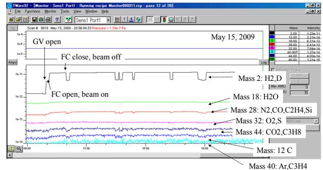
Figure 2: Measured data from the Q-mass analyzer.
