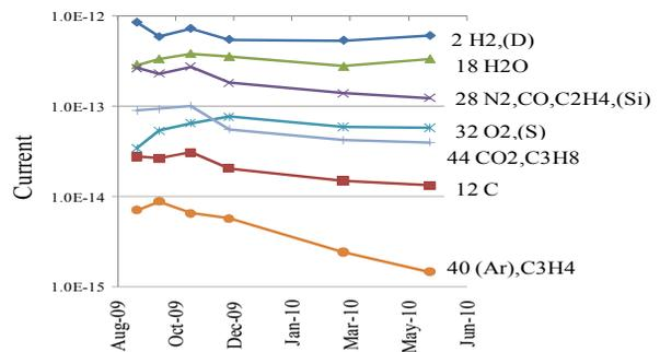
Figure 6: Long term residual gas components during conditioning. Note that the duty factors and voltage levels are not the same as the condition has been getting better.
