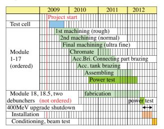
Figure 1: Schedule of the Linac 400 MeV energy upgrade. The 17 ACS modules are already ordered; each fabrication step of 17 modules (first, second, final machining etc.) proceeds in parallel. The first module will be finished in the summer of 2010.
