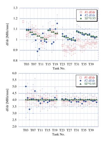
Figure 3: Coefficient  $\alpha$  of the accelerating cell (above) and the coupling cell (bottom). The red squares are coefficients of the first tuning, the blue diamonds are of the second tuning, and the green triangles show the 0.95 times of the SU-PERFISH calculation.
