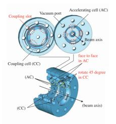
Figure 2: Exploded view of the Annular Coupled Structure (ACS) used at the J-PARC. The four coupling slots connect the Accelerating Cell (AC) and the annular ring type Coupling Cell (CC).
