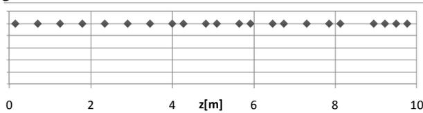
Figure 3: Tuners positions along the RFQ.
