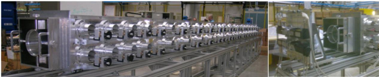
Figure 1: The aluminium model of the IFMIF RFQ set up for measurements at LNL (left) and the bead pulling system (right) .
