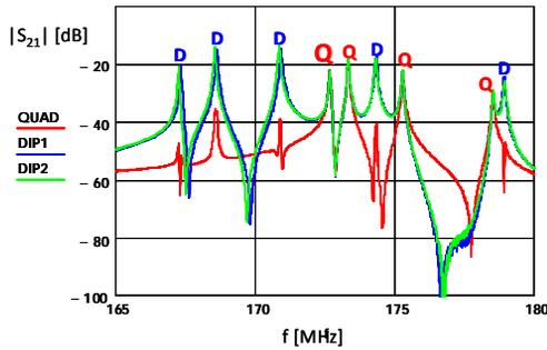
Figure 2: Mode spectra of the Aluminum RFQ.
