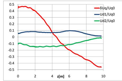
Figure 4: Perturbative components of the RFQ, with tuners inserted at 30 mm depth.
