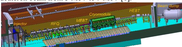
Figure 1: General Layout of the IFMIF-EVEDA accelerator in the Rokkasho vault
