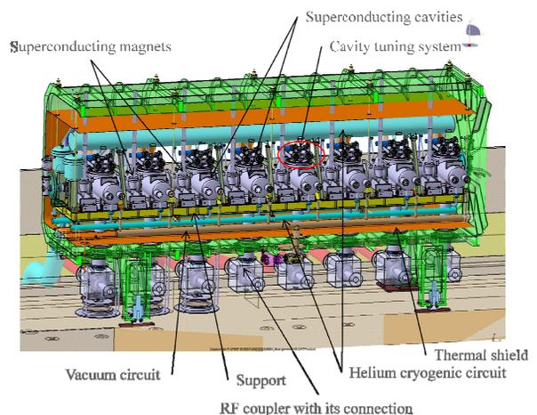
Figure 2: Cryomodule section view
