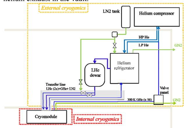
Figure 5: Principle scheme of the cryogenic systems
