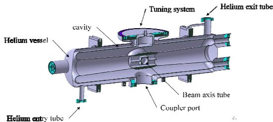
Figure 3: HWR section view
