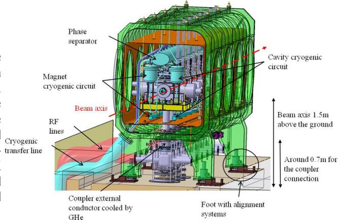
Figure 4: Cryomodule cryogenics and interfaces
