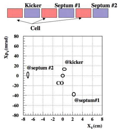
Figure 4: Phase space motion of extracted beam in 2septum option.
