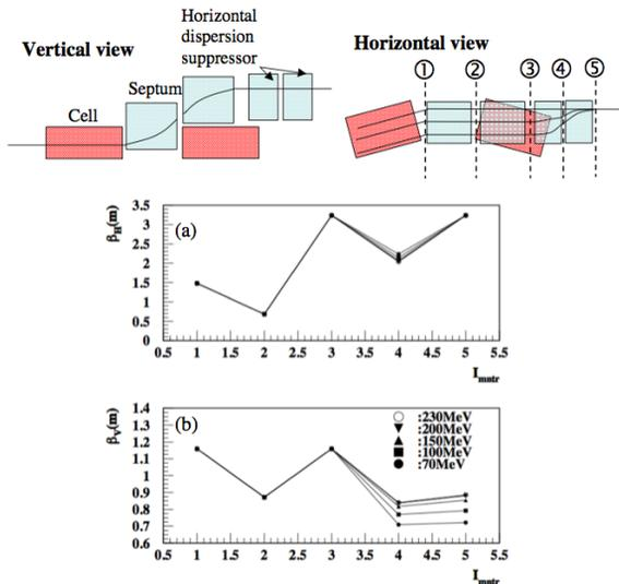
Figure 3: Beta function in extraction and matching section (a): $\beta_H$ , (b): $\beta_V$ .
