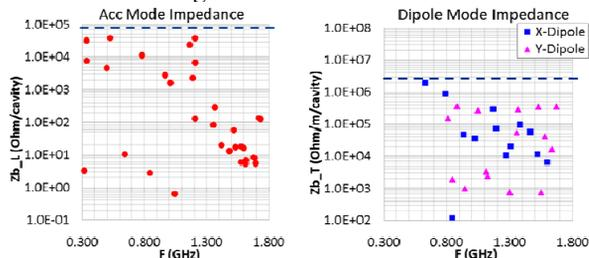
Figure 8: Left: impedance of accelerating modes; Right: impedance of dipole modes. The horizontal dashed lines are the impedance limits for the LHC crab cavity.
