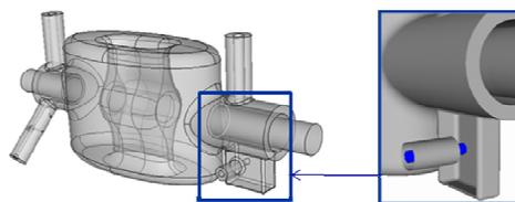
Figure 9: Input coupler for the HWSR crab cavity.
