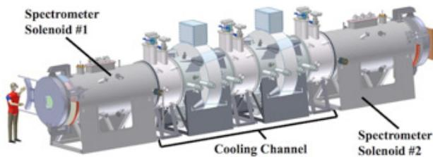
Figure 1: MICE cooling channel 3D CAD image.
