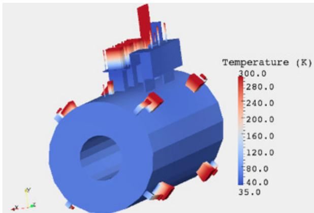
Figure 4: Model temperature distribution at full current.
