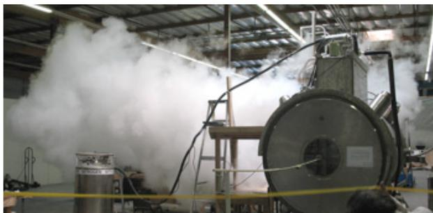
Figure 7: Quench during spectrometer solenoid training.
