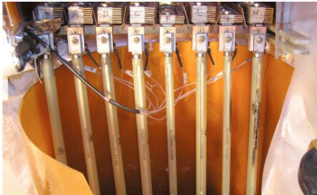
Figure 6: Burned out HTS lead (right side).
