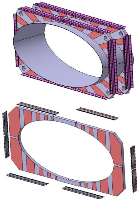
Figure 4: The vacuum chamber adapted for contact cooling. Only 2 periods are shown. The copper paths are given in red.
