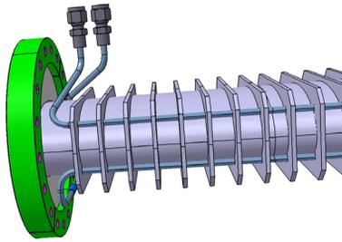
Figure 1: Vacuum chamber with mechanical stabilising ribs and the additional cooling scheme on the beam pipe.
