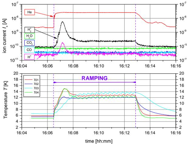
Figure 2: Chamber temperatures and partial pressure conditions during magnet ramping with 4 T/s between 0 -  $B_{max}$  - 0 with a repetition rate of 0.5 Hz.
