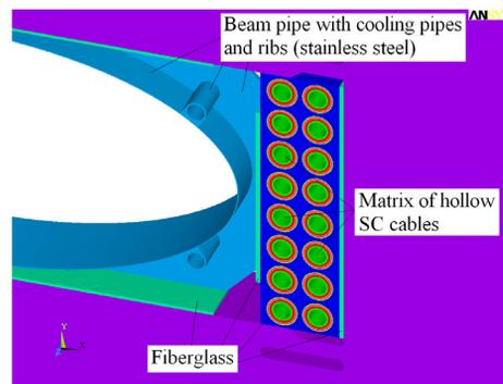
Figure 3: FEM magnet – vacuum chamber model.
