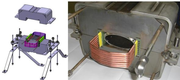
Figure 5: The vacuum chamber direct cooling test setup.
