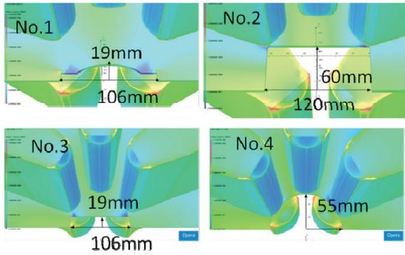
Figure 4: Four shapes of steel shield.
