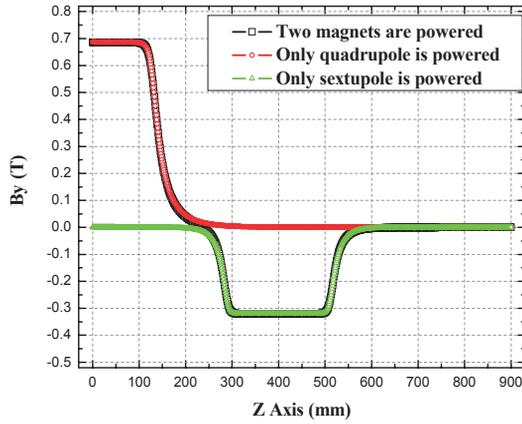
Figure 2: Distance between centers of quadrupole and sextupole magnets is 400 mm. The vertical field component ( $B_y$ ) lies along the beam axis ( $x=40\text{mm}$ ,  $y=0$ ) in three cases.
