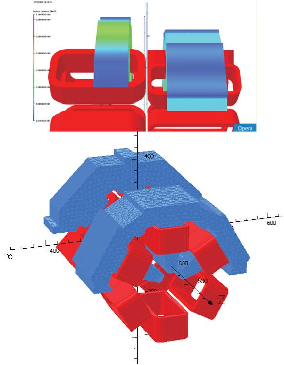
Figure 1: One tight case of the TPS quadrupole and sextupole magnets for study of the crosstalk effect.
