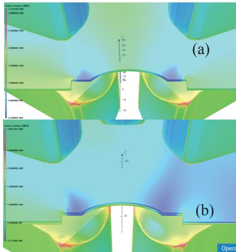
Figure 5: Varied thickness of No.1 steel shield, (a) one shield of 5 mm (b) two shields of thickness 2.5 mm separated 1 mm.
