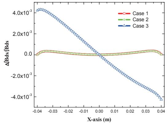
Figure 3: Field homogeneity of the integral fields on the transverse x-axis;  $\Delta[\int B ds / \int B ds] = [\int B(x) ds - (B_0 + B_1 x)] / \int B(x) ds$ .
