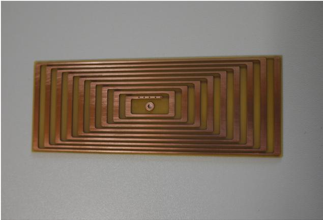
Figure 3: Printed Circuit board for the steerer magnet. An equivalent spiral pattern is etched onto the backside.
