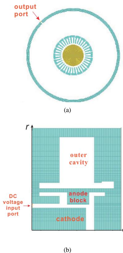
Figure 1: (a) Sectional view of the coaxial magnetron in the  $r\theta$  plane. (b) Sectional view of the coaxial magnetron in the  $rz$  plane.
