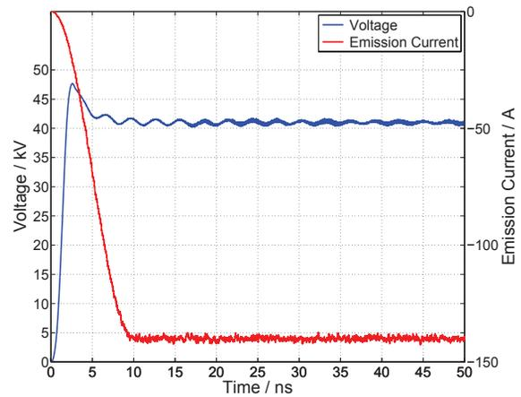
Figure 3: Applied DC voltage and emission current from the cathode
