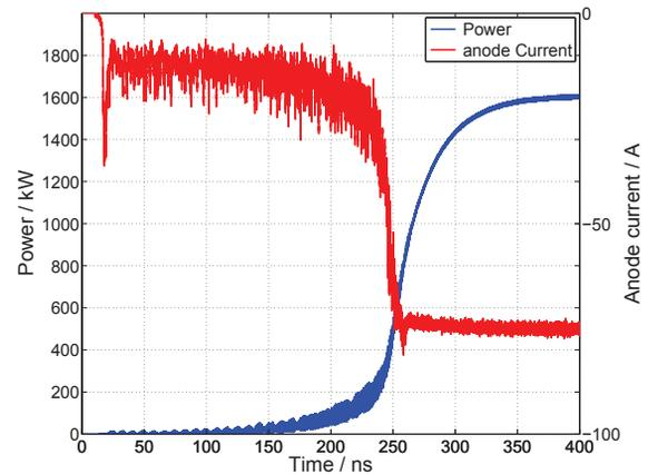
Figure 7: Temporal output power and current collected on the anode
