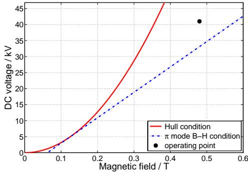
Figure 2: Hull cutoff condition and Buneman-Hartree resonance condition of the magnetron
