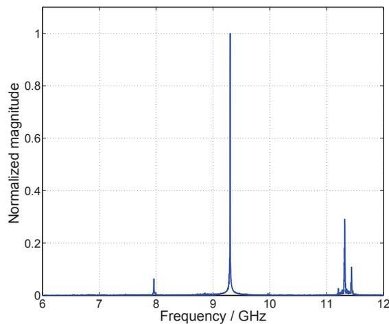
Figure 6: A frequency spectrum obtained from Fourier transformation of the time-varying electric fields
