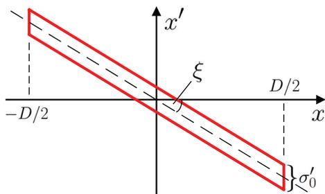
Figure 2: A typical  $x-x'$  distribution after collimation
