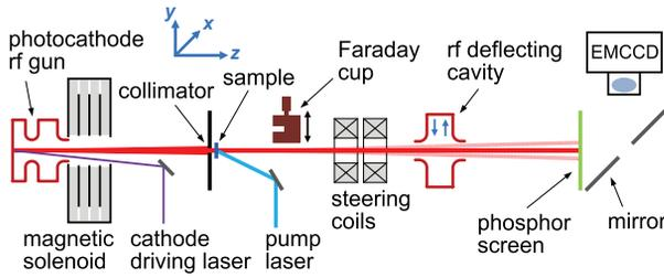
Figure 1: Schematic of the MeV UED system
