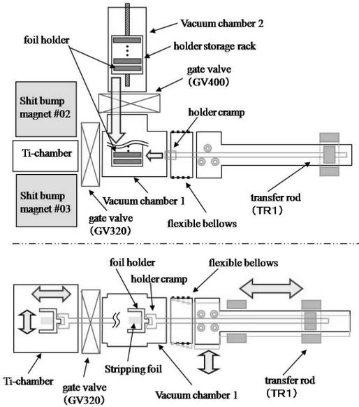
Figure 2: Hardware components of the drive system.
