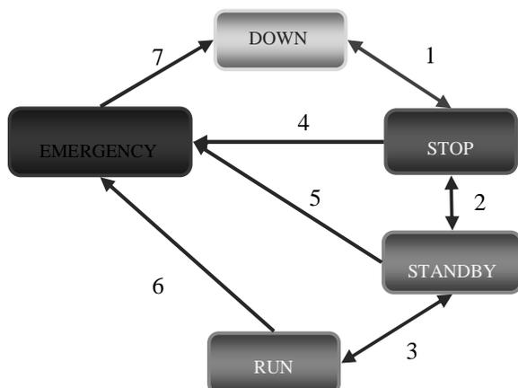
Figure 5: The machine status transition diagram for the charge exchange device.
