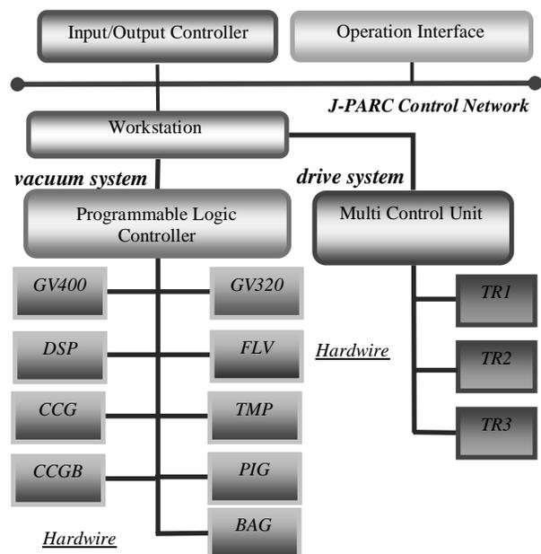
Figure 1: Components of control system for the charge exchange system.
