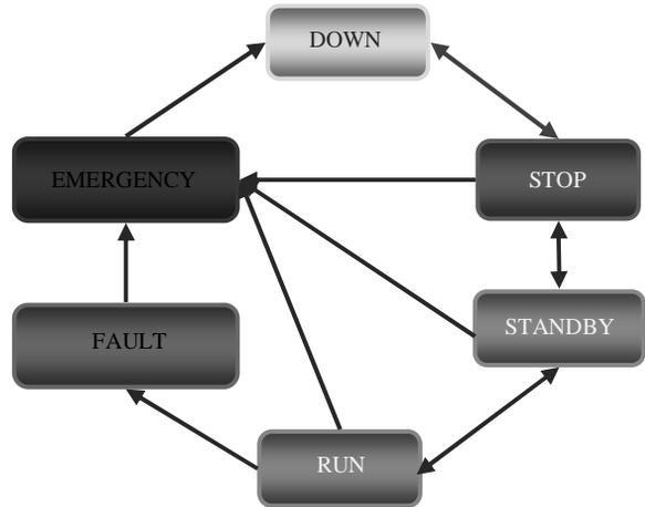
Figure 4: The machine transition cycle.
