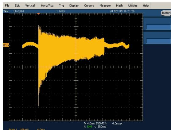
Figure 1: Output signals from bunch monitor of the main ring.
