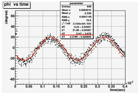
Figure 6: Measured synchrotron oscillation phase.
