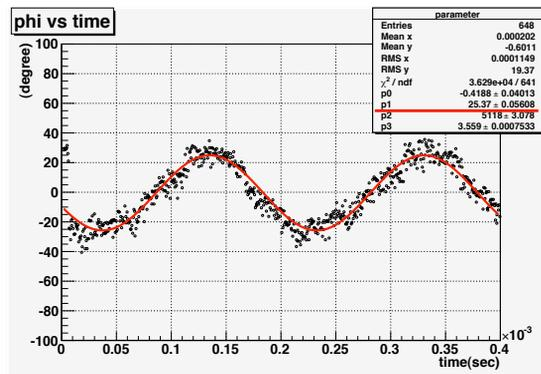
Figure 7: Measured synchrotron oscillation phase before optimization.
