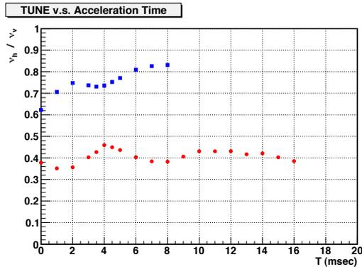
Figure 3: Measured betatron tunes as a function of acceleration time. Blue squares indicate decimal part of the horizontal betatron tune  $\nu_h$  and red circles indicate decimal part of the vertical betatron tune  $\nu_v$ .
