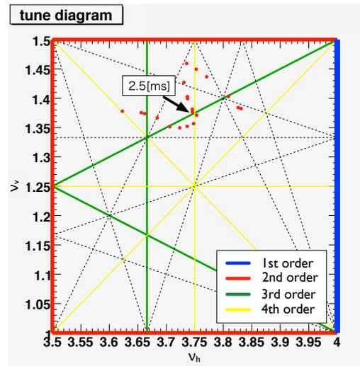
Figure 4: Measured betatron tunes diagram in the main ring.
