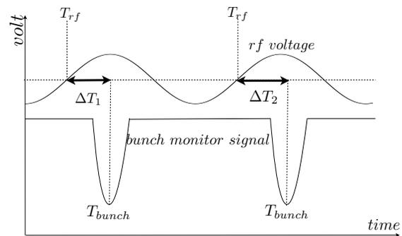
Figure 5: Concept of synchrotron oscillation phase measurement.
