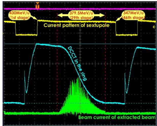
Figure 6: A current pattern for the sextupole magnets (yellow), the DCCT in the ring (blue), and the measured beam current of the extracted beam (green). The beam energy of the extracted beam is 379.5 MeV/u.
