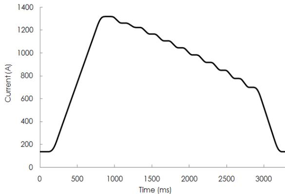
Figure 2: A current pattern for the main-bending magnets in the ring as a function of time. The currents of the 11 flattops correspond to the beam energies of 430, 400, 380, 350, 320, 290, 260, 230, 200, 170, and 140 MeV/u.
