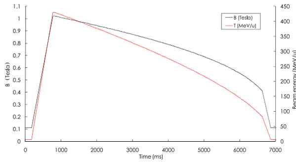
Figure 4: A magnetic-field pattern of the main-bending magnets for the ring and corresponding beam energy as functions of time for the 146 flattop pattern.
