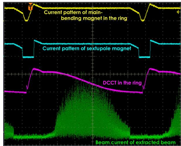
Figure 3: Current patterns for the main-bending magnets (yellow), the sextupole magnets (blue), DCCT in the ring (pink), and the measured beam current of the extracted beam (green). The 6th flattop, corresponding to the beam energy of 290 MeV/u, was extended, and the beam was extracted during that flattop.
