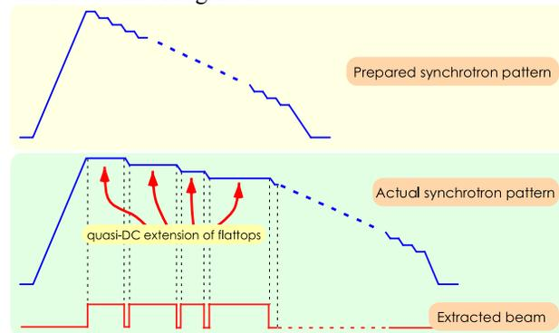
Figure 1: A schematic drawing of an operation pattern for the synchrotron ring. The operation pattern has a stepwise flattop; each flattop can be extended, and the beam could be extracted from the synchrotron ring during any of these flattops.
