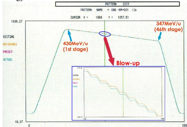
Figure 5: A current pattern of the main-bending magnets in the ring. The currents of the flattops for the 46 stages correspond to the energies between 430 and 347 MeV/u.
