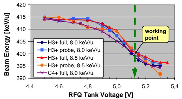
Figure 4: RFQ output beam energy as function of the scaled tank voltage for different ion beams (see text).
