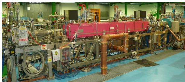
Figure 2: Complete linac with RFQ (right), IH linac (center), and foil stripper section (left).
