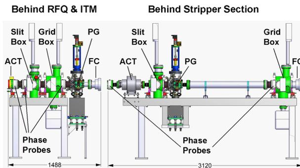
Figure 3: Beam diagnostics test benches used during beam commissioning of RFQ (left) and IH-DTL (right). Beam direction from left to right. ACT = fast beam Current Transformers, FC = Faraday Cup, PG = Profile Grid.
