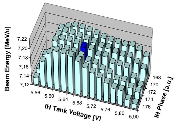
Figure 5: Beam energy of C<sup>4+</sup> beams measured behind the IH linac as function of the scaled tank voltage and phase.
