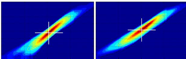
Figure 7: Horizontal (left) and vertical (right) proton beam emittances measured ~1 m behind the stripping foil. Axis ranges are  $\pm 10$  mm and  $\pm 8$  mrad, respectively.
