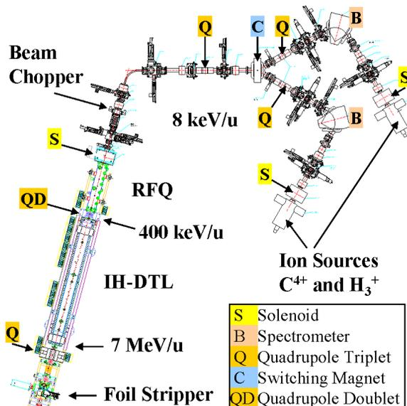
Figure 1: Layout of the CNAO injector.
