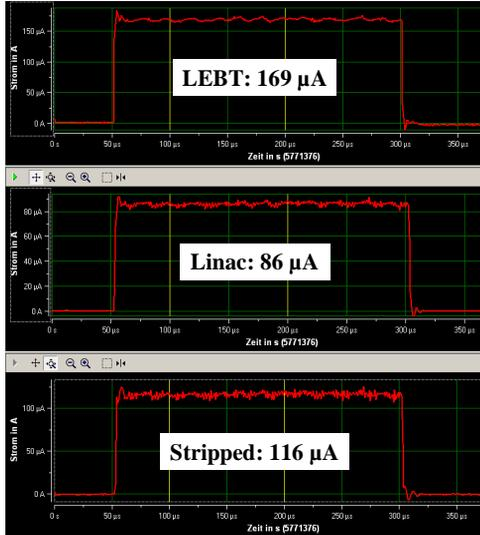
Figure 6: Measured  $\text{C}^{4+} / \text{C}^{6+}$  beam currents.
