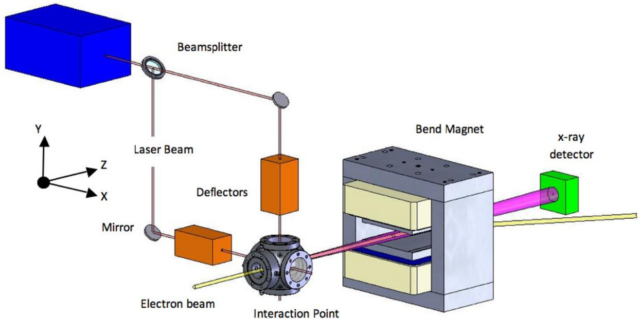
Figure 1: A schematics of LWS measurement system.
