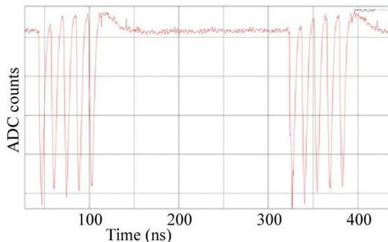
Figure 6: digitized waveform from current readout system. The display shows 5 bunches with 14ns separation in trains with 280ns separation.
