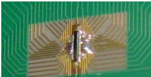
Figure 2: diode array
