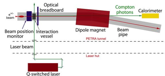
Figure 2: Overview of the LW setup [1].
