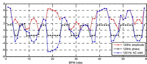
Figure 9: 120 Hz horizontal BPM amplitude, phase and AC orbit
