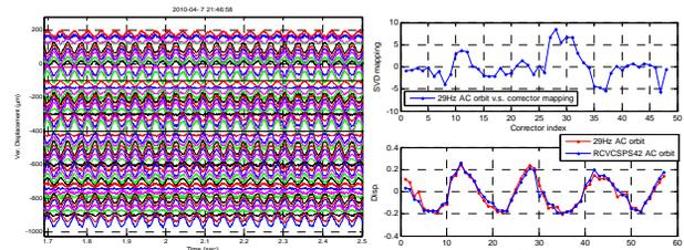
Figure 14: (a) BPM vertical data with strong 29.2Hz noise (b) Correlation between 29.2 Hz vertical AC orbit versus all vertical correctors. Max correlation is RCVCS42.
