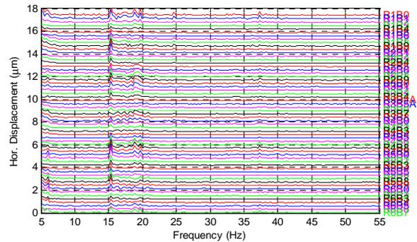
Figure 2: Horizontal orbit motion spectrum. The noise spreading between 15~25 Hz is correlated to the ground vibration.
