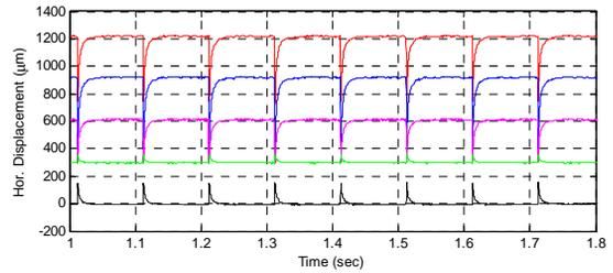
Figure 7: Orbit motions of 5 BPM during injection caused by kicker and septum.
