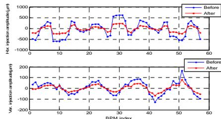
Figure 8: Orbit distortion caused by septum leakage before and after septum shielding.
