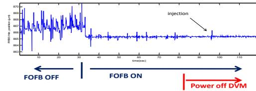
Figure 13: R1BPM3 horizontal position change for fast orbit feedback system on/off and DVM on/off.
