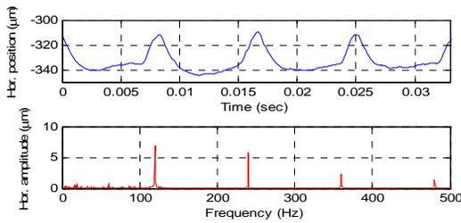
Figure 4: Orbit motion due to the ill superconducting wiggler power supply.
