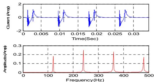
Figure 3: Superconducting wiggler power supply current readings and its spectra amplitude
