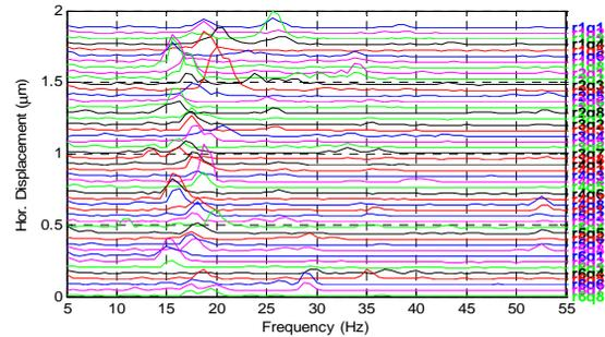
Figure 1: Quadrupole horizontal vibration
