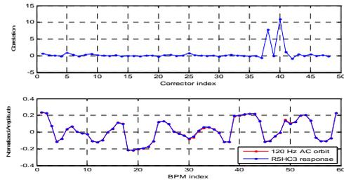
Figure 10: The above figure is correlation between 120 Hz horizontal AC orbit versus all horizontal correctors. The below one shows the AC orbit and its most relevant corrector (R5HC3) response.
