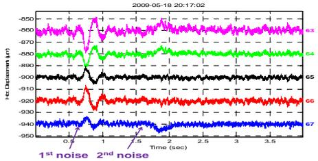
Figure 11: Horizontal orbit motions of 5 BPM for 4.8 sec disturbed source.
