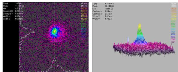
Figure 6: 2D (a) and 3D (b) image of THz using IR-CCD camera. CCD size is 12.4 mm  $\times$  12.4 mm.
