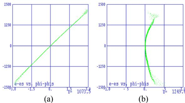
Figure 3: PARMELA simulation result for bunch distribution in phase space before (a) and after (b) chicane. The horizontal axis is distance between a synchronous particle and arbitrary particles in degrees (1 degree is about 1 ps) and the vertical axis is energy difference between a synchronous particle and arbitrary particles in KeV.
