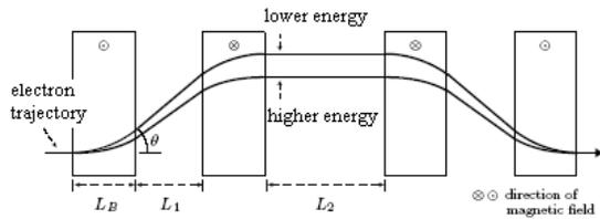
Figure 2: Chicane (rectangles) and electron beam trajectory.
