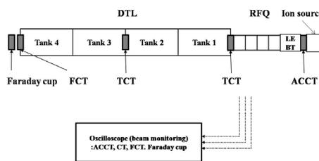
Figure 2: Diagram of beam current transformer and measurement system for the 20-MeV Linac.
