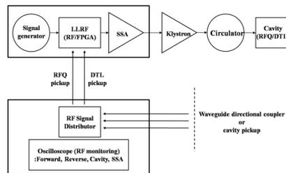
Figure 1: Diagram of RF system for the 20-MeV Linac.
