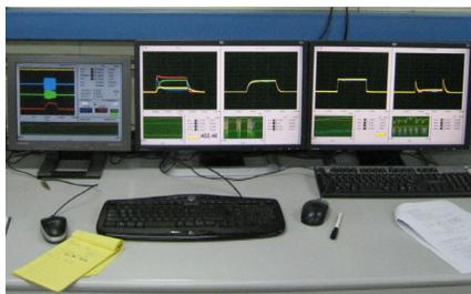
Figure 4: Display monitors of RF and BCM using LabVIEW user interface.
