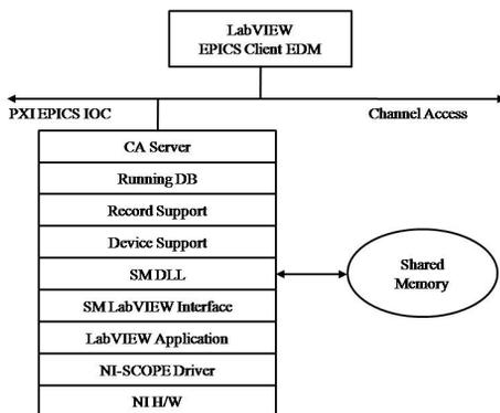
Figure 9: Schematic diagram of software modules using PXI NI-SCOPE and LabVIEW EPICS IOC scope
