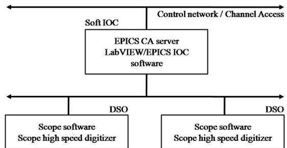
Figure 5: Diagram of EPICS based software structure.
