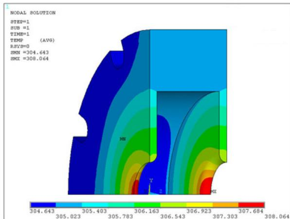
Figure 5: Temperature [K] distribution on the cavity
