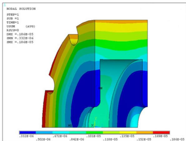
Figure 6: Structural deformation [m] of the cavity
