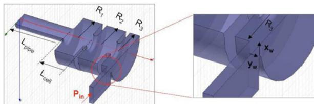
Figure 1: Schematic view of a quarter of the deflector
