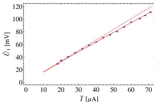
Figure 2: Measured pick-up signal as a function of the current of a silicon beam having a velocity of  $\beta = 0.0872$ .
