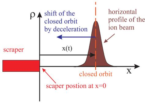
Figure 3: Principle of the profile measurements by deceleration of the ion beam towards the scraper.
