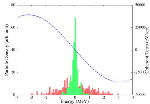
Figure 1: Initial particle distribution (red) and after 400 sec cooling (green). The coherent term (right scale) is obtained with stochastic cooling parameters with gain=110 dB.
