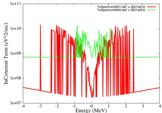
Figure 4: Diffusion term including the Schottky noise, thermal noise and IBS effects. Horizontal scale is proton energy and vertical scale the diffusion term. Red line shows the initial, and green line after 400 sec cooling.
