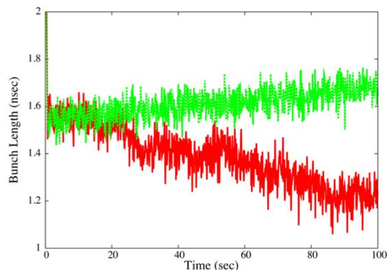
Figure 5: The simulated evolution of beam bunch length with time. Red line shows the case with stochastic cooling and green line without cooling.
