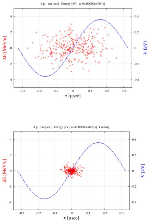
Figure 2: Numerical simulation results. Particle distribution (red points) at time=0 sec (top) and at 400 sec (bottom). The horizontal scale is time (micro sec) and the vertical scales the energy (left scale) and RF voltage. (right scale).
