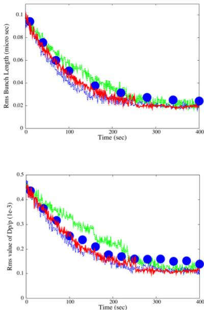
Figure 3: Evolution of bunch length (top) and  $Dp/p$  (bottom) with time. Red: simulation results for gain=110dB, green for 107dB and blue for 112dB, respectively. Blue points are measured ones.
