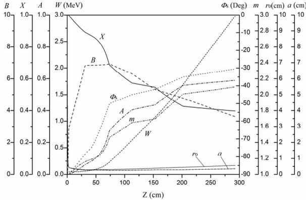
Figure 2: Various parameters of the CPHS RFQ versus longitudinal position.
