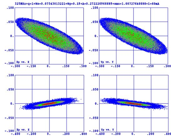
Figure 5: Particle distribution in the transverse plane x-y at the entrance and exit of the RFQ.
