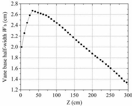
Figure 3: Vane base half-width versus longitudinal position.
