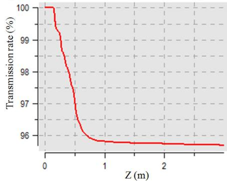
Figure 6: Beam transmission versus position by the code of TOUTATIS.
