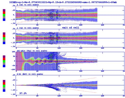
Figure 4: Beam dynamics in the RFQ by PARMTEQM for the input current of 60mA.
