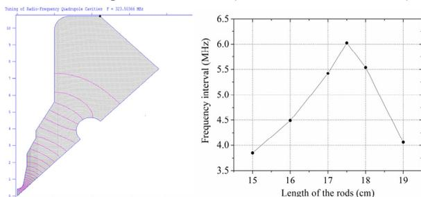
Figure 8: Design of the position and length of the dipole-mode stabilizer rods.
