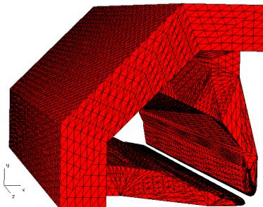
Figure 7: 3D model established by the MAFIA code to optimize the undercut design.
