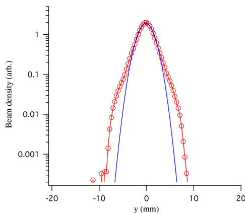
Figure 3: Typical beam profile measured at the SDTL exit with 30 mA peak current.
