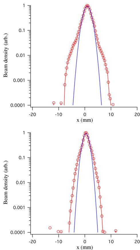
Figure 4: Typical beam profile measured at the SDTL exit with 15 mA peak current. Before (top) and after (bottom) the longitudinal matching at the DTL entrance.
