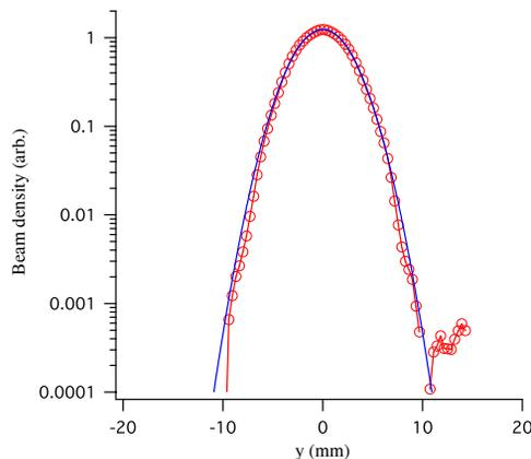
Figure 2: Typical beam profile measured at the DTL exit with 30 mA peak current. Red circle: measurement, blue line: Gaussian fit. The same notation is adopted in Figs. 3, and 4.
