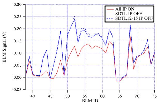
Figure 1: BLM raw signals with different IP settings. With all IP's on (red), IP's in the SDTL section off (blue solid), and IP's in the downstream quarter of the SDTL section off (blue broken). BLM #40 corresponds to the one at the SDTL end, and BLM #44 to #65 correspond to those in the future ACS section.
