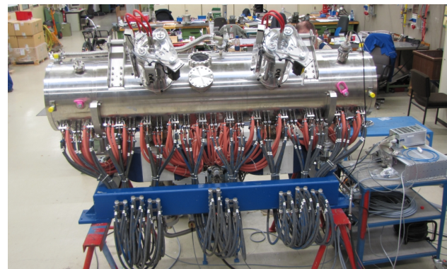
Figure 2: New RFQ during assembly of the water and prevacuum connections.
