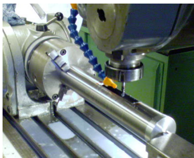
Figure 3: Photograph of the manufacturing of the movable electrode of the Einzellens.
