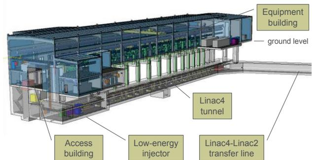
Figure 2: The Linac4 installations.
