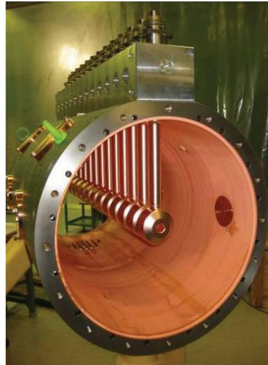
Figure 4: DTL prototype.
