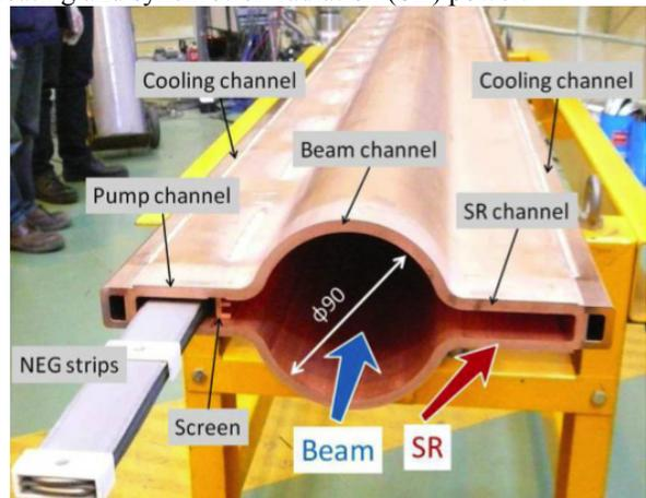
Figure 11: Antechamber for the LER arc-sections.
