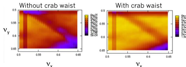
Figure 5: Illustration of suppression of X-Y betatron resonance by crab waist. (Note: simulation is for SuperKEKB.)
