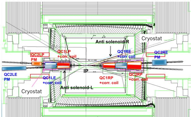
Figure 8: SuperKEKB IR. The permanent magnets (QC2LP, QC2LE and QC2RE) are located further from the IP than the superconducting magnets.
