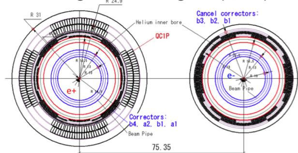
Figure 9: Design of superconducting IR quadrupole for the LER, with the leakage field cancelled by correction coils wound on the HER beam pipe.
