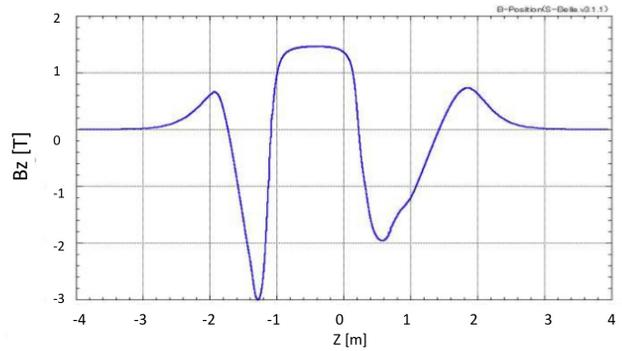
Figure 10: Solenoid field profile along the Belle-II axis.
