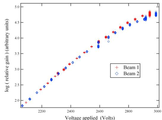
Figure 6: Calibration of PMT gain curve with beams
