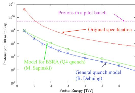
Figure 2: Quench threshold predictions as a function of the beam energy
