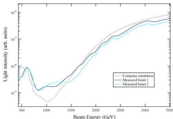
Figure 7: Evolution of the Synchrotron light intensity with beam energy
