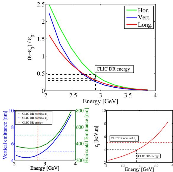
Figure 4: Relative difference of the emittances in the horizontal (blue), vertical (green) and longitudinal (red) planes with the energy (top). Steady state horizontal, vertical and longitudinal emittances on energy (bottom).
