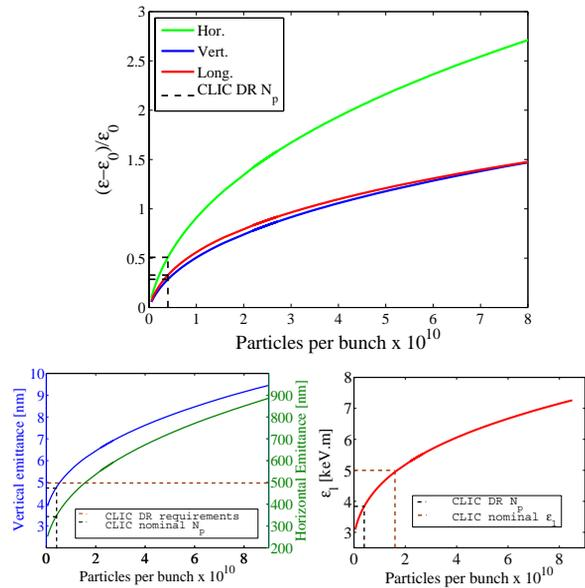
Figure 2: Scaling of the relative difference of the steady state and the equilibrium horizontal, vertical and longitudinal emittance with the bunch charge (top). The CLIC DR nominal bunch charge is indicated with dashed black lines. The dependence of the steady state emittances, horizontal and vertical (bottom, left) and longitudinal (bottom, right). The CLIC DR emittance nominal values are indicated with brown dashed lines and the nominal bunch charge with dashed black lines.
