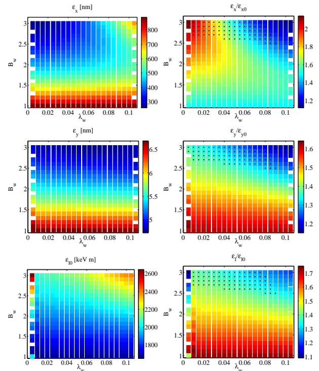
Figure 5: Scaling of the extracted emittances with the wiggler field and period. In the left plots the extracted emittances are shown, while in the right ones the ratio between the extracted and the zero current emittances. The black dots indicate solutions where all the emittance requirements are met. The longitudinal emittance is kept constant.
