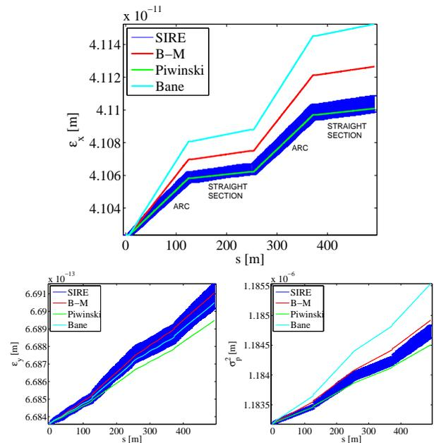
Figure 1: The one turn behavior of the horizontal emittance (top), vertical emittance (left, bottom) and energy spread (right, bottom), starting from the zero current values, as they are computed by SIRE (dark blue) and BM (red), Piwinski (green) and Bane (light blue) formalisms. In the case of SIRE, the  $1\sigma$  errorbars are also shown.
