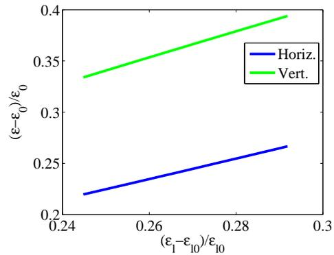
Figure 3: Dependence of emittance relative difference in the horizontal (green) and vertical (blue) plane on the relative difference in the longitudinal plane.
