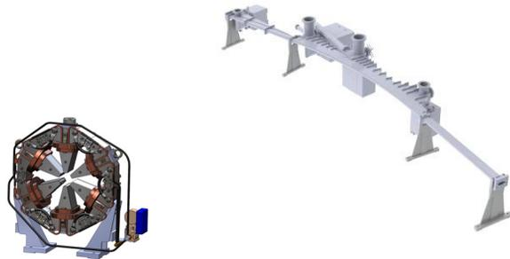
Figure 7: (a) 3D model SR sextupole. (b) 3D model SR arc vacuum chamber.
