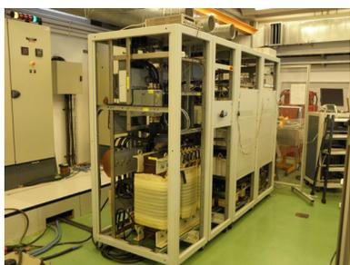
Figure 4: The dipole power converter under construction.
