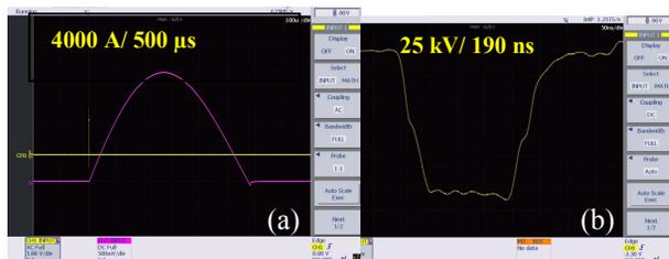
Figure 3: (a) Extraction septum magnet current waveform. (b) Extraction kicker magnet pulser waveform.
