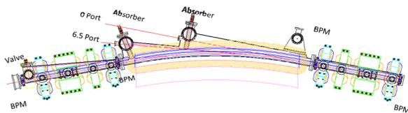
Figure 6: One Storage Ring arc chamber assembly.
