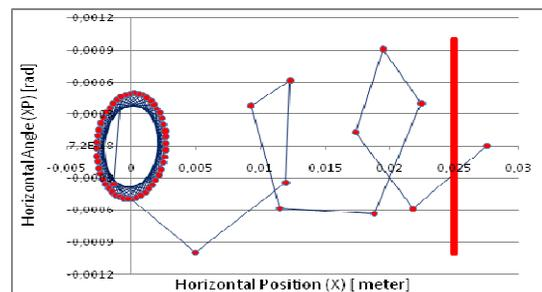
Figure 2: Phase space after tracking one particle for 60 turns at the injection point (septum sheet in red).
