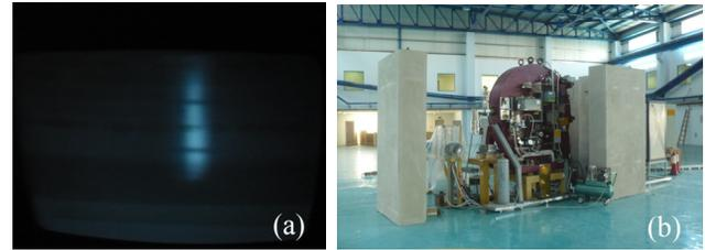
Figure 1: (a) The first beam from SESAME Microtron, (b) The temporary shielding wall around the Microtron.
