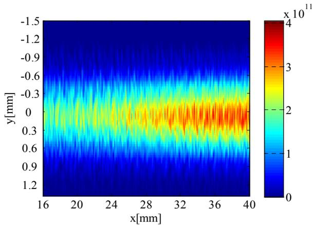
Figure 2: Particle density in p+ / mm<sup>2</sup> for a beam sweep over the TCDSA front surface, 7 TeV.
