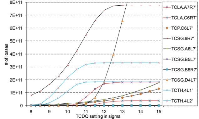
Figure 4: Losses for the TCTH and TCLA collimators for the 1 MKD case, 7 TeV, 10 orbit seeds.
