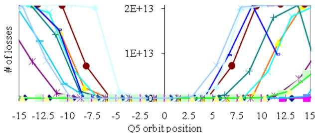
Figure 7: Total losses in the extraction channel for extractions with orbit offset at Q5, 450 GeV.
