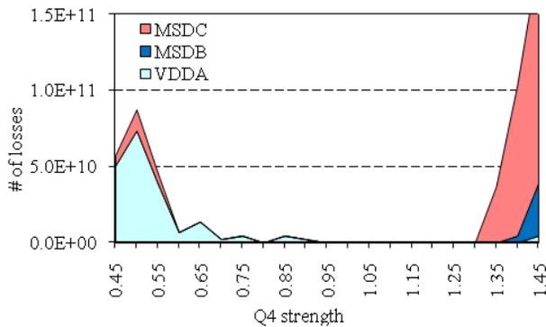
Figure 6: Losses in the extraction channel (TCDS not shown) for Q4 strength failures, 450 GeV.
