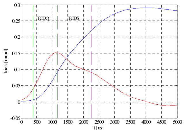
Figure 1: MKD kick waveform (blue) and its first derivative (red) with markers when sweeping over the TCDQ (green) and TCDS (magenta) apertures.
