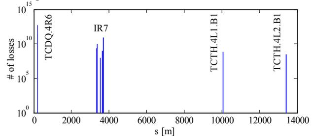
Figure 5: Loss pattern for an asynchronous dump at 7 TeV, prefire case, and TCDQ at  $8 \sigma$ .
