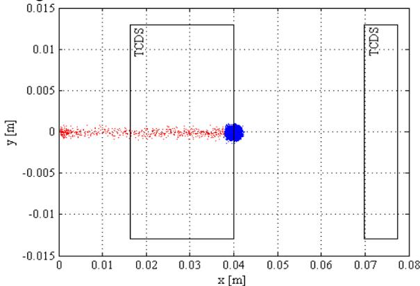
Figure 3: Beam sweep over the TCDS Aperture for 7 TeV and three missing kickers. Particles within the abort gap are indicated in red.
