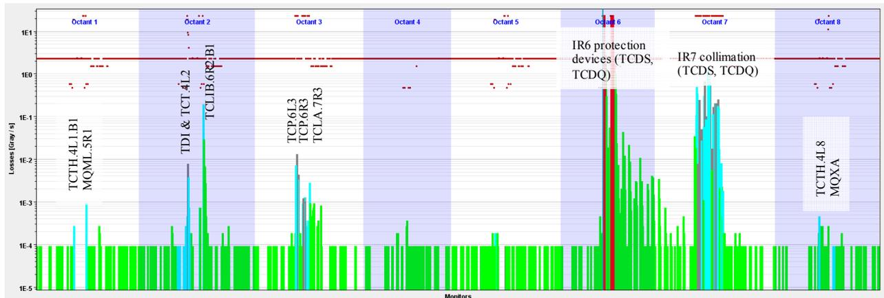
Figure 8: BLM signals during a provoked asynchronous dump at 450 GeV,  $1 \times 10^{11}$  p<sup>+</sup> total intensity.
