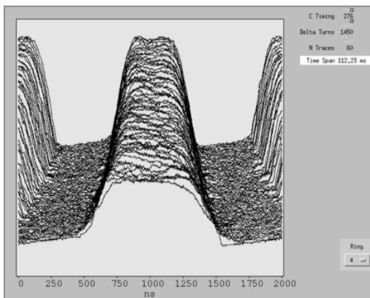
Figure 2: Mountain range plot after beam capture.
