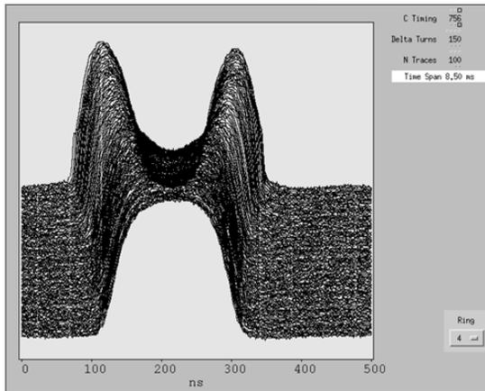
Figure 3: Mountain range plot of the splitting process.
