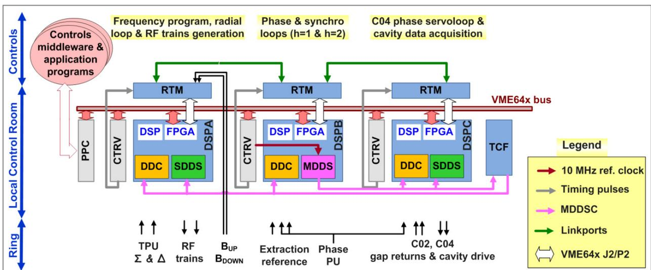
Figure 1: PSB test LLRF - schematic view [3]. Keys: MDDS – Master Direct Digital Synthesiser (DDS); SDDS - Slave DDS; DDC – Digital Down Converter; MDDSC – Tagged Clock; TCF – Tagged Clock Fanout; TPU – Transverse Pick-Up; CTRV – Timing Receiver Module; PPC – Power PC;  $B_{up}$ ,  $B_{down}$  – measured magnetic field.
