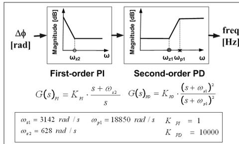
Figure 4: Extraction synchro corrector - transfer function.
