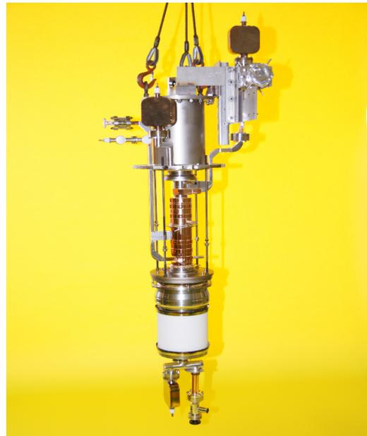
Figure 3: The XL5-1 klystron ready to ship.
