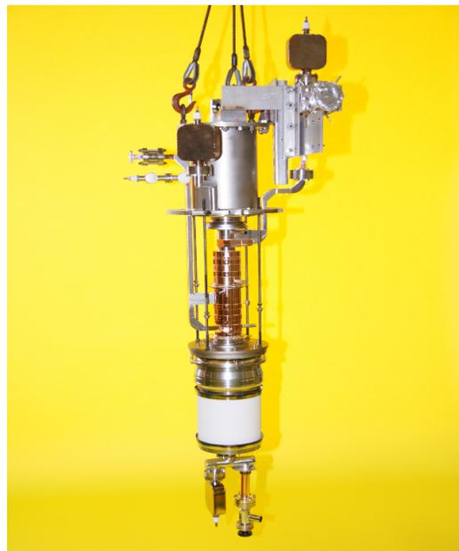
Figure 3: The XL5-1 klystron ready to ship.
