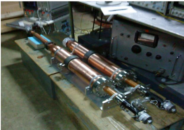
Figure 5: SLED-I type pulse compressor at cold testing
