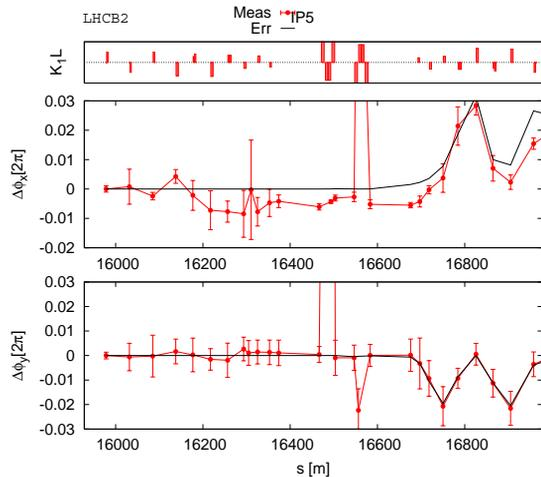
Figure 6: The plot shows the horizontal total phase advance above and the vertical below. The total phase is the difference between propagated phase advance and ideal model phase advance. From the plot below it is clear that there is an error at around 16700 m.
