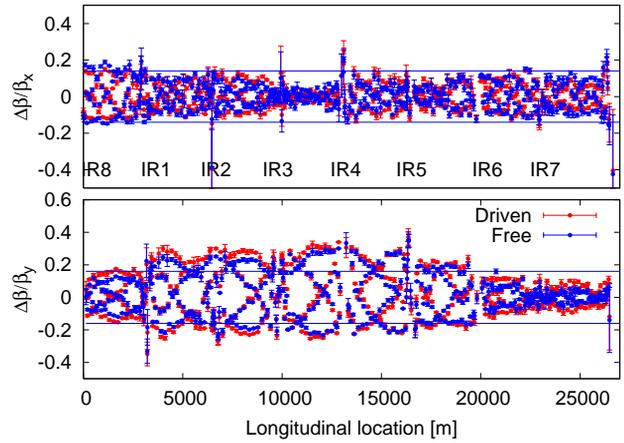
Figure 4: Plot showing the difference between the driven beta-beat from the ac-dipole (blue) and the calculated free beta-beat (red), horizontal plane above and vertical plane below
