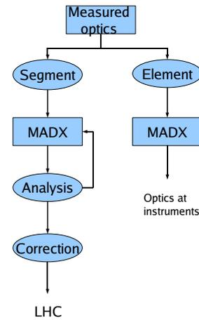
Figure 5: Flow diagram showing the steps done for segment-by-segment. Segment-by-segment uses the measured optics, such as phase,beta,dispersion and coupling to calculate for a segment or a single element.
