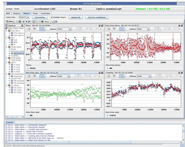
Figure 1: Screenshot of the graphical user interface for the LHC. This tab is showing a typical result of the analysis. Clockwise you have a plot of the horizontal phase advance, horizontal beta-beat from phase, vertical beta-beat from the amplitude and the difference resonance coupling term.
