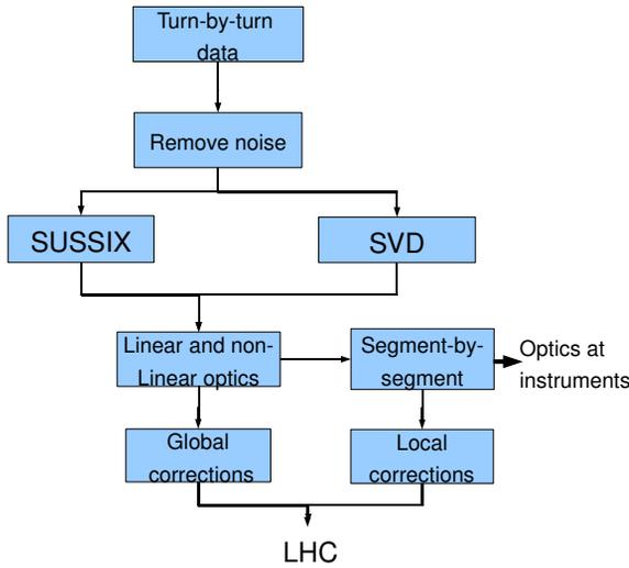
Figure 2: Flow diagram showing the steps done during operation. Turn-by-turn data is acquired using either a single kick or ac-dipole. The turn-by-turn data is then decomposed in Fourier basis. From the output the linear and non-linear optics are calculated. When a large discrepancy is observed segment-by-segment can be used to identify local sources. From this a local correction or when only small distributed errors a global correction can be calculated and send to the machine.
