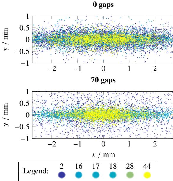
Figure 1: Transverse distribution of the macro-ions zoomed at the center of the beam pipe, after 24  $\mu$ s, for the machine configuration with 0 and 70 gaps. The legend shows the correspondence between the dot colors and the ion masses in atomic mass units.
