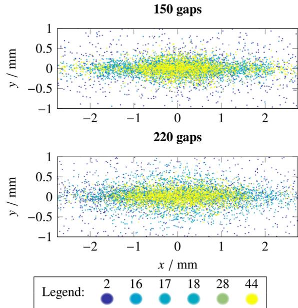
Figure 2: Transverse distributions of the macro-ions zoomed at the center of the beam pipe, after 55  $\mu$ s, for the machine configuration with 150 and 220 gaps. The legend shows the correspondence between the dot colors and the ion masses in atomic mass units.
