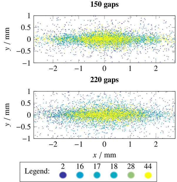
Figure 2: Transverse distributions of the macro-ions zoomed at the center of the beam pipe, after 55  $\mu$ s, for the machine configuration with 150 and 220 gaps. The legend shows the correspondence between the dot colors and the ion masses in atomic mass units.
