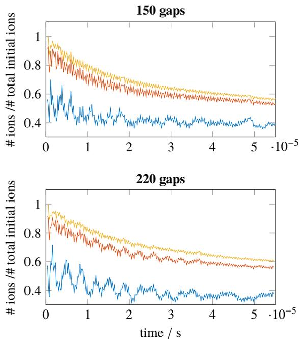
Figure 4: Time evolution of the number of ions inside the elliptic cylinder  $C_1$  (blue),  $C_2$  (red),  $C_3$  (yellow), for the fill patterns with 150 and 220 gaps.
