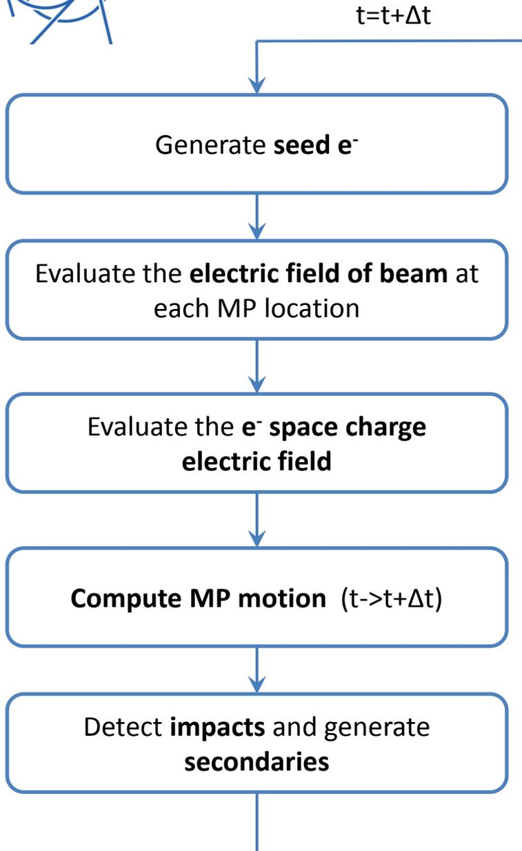
PyECLOUD is a **2D macroparticle (MP) code** for the simulation of the **electron cloud build-up** with:
