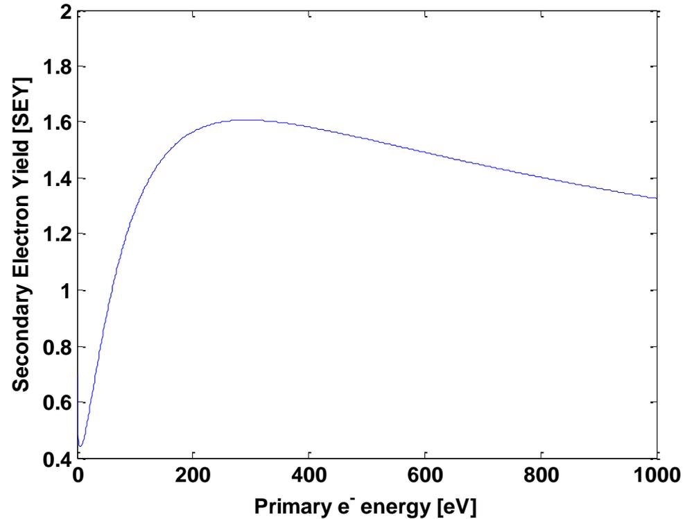
The **Secondary Electron Yield** of the chamber's surface is basically the ratio between emitted and impacting electrons and is function of the energy of the primary electron.
