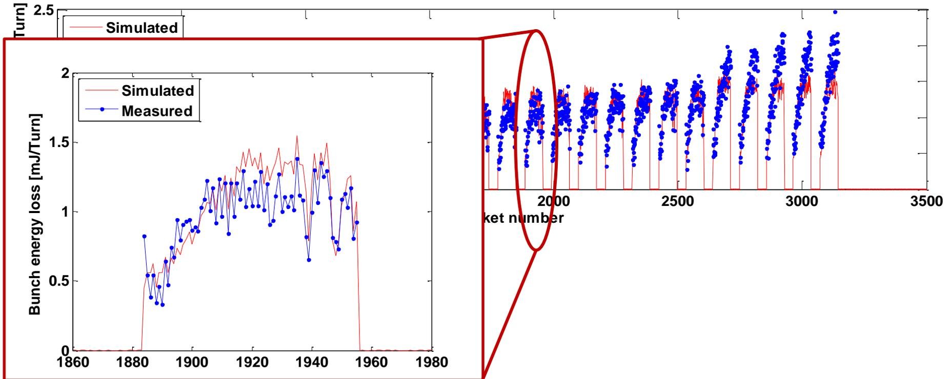
Simulation results could be **benchmarked with measured bunch by bunch energy loss**
