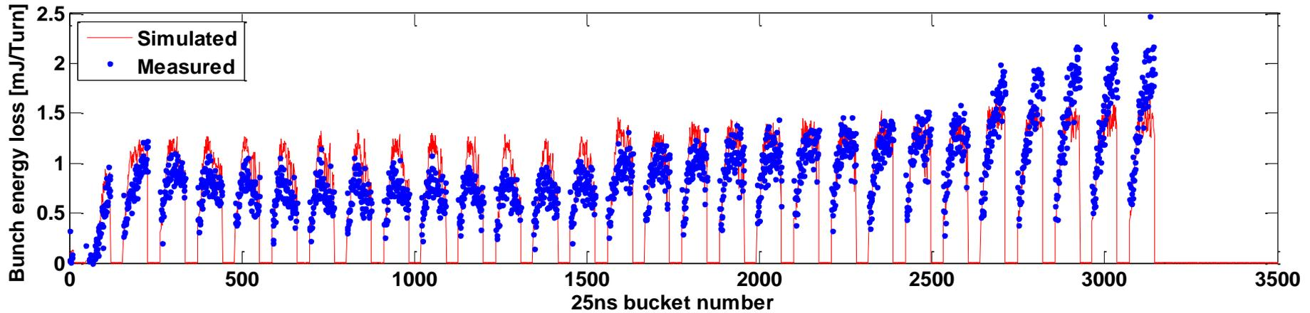
Simulation results could be **benchmarked with measured bunch by bunch energy loss**
