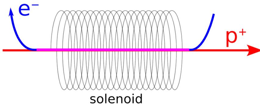
Compensate beam-beam kicks by kicks of an electron beam of comparable charge density distribution at identical betatron phase (not necessarily full compensation)
