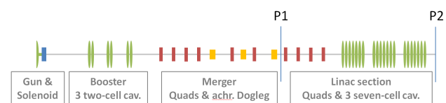
Figure 2: BERLinPro Injector elements used for the optimization: gun, booster and main linac cavities (light green), the gun solenoid (dark green), the three merger bends (yellow) and ten quadrupoles (red). The beam line and thus the ASTRA run is split at P1, right after the last merger bend, where the beam has changed its direction.
