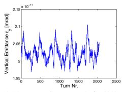
Figure 4: Almost no emittance growth after 2048 turns with  $\rho_e = 5 \cdot 10^{11} \text{ N}_e/\text{m}^3$ .
