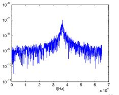
Figure 5: Vertical tune spectra for  $\rho_e = 5 \cdot 10^{11} \text{ N}_e/\text{m}^3$
