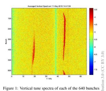
Figure 1: Vertical tune spectra of each of the 640 bunches with 8ns spacing, measured on May 11, 2010 [1]. The total beam current was 62 mA. The red color represents the sidebands and the vertical betatron frequency of 38kHz is green. (Courtesy of R. Wanzenberg.)
