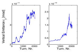
Figure 6: Emittance growth after 2048 turns for  $\rho_e = 2 \cdot 10^{12} \text{ N}_e/\text{m}^3$  (left) and for  $\rho_e = 5 \cdot 10^{12} \text{ N}_e/\text{m}^3$  (right).
