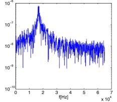
Figure 7: Horizontal tune spectra for  $\rho_e = 2 \cdot 10^{12} \text{ N}_e/\text{m}^3$ .
