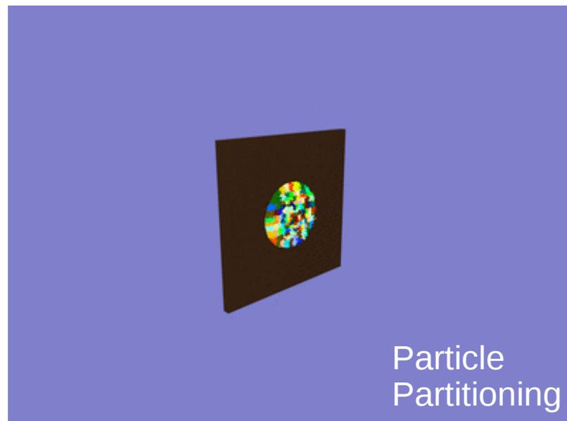
Example: LCLS RF gun, colors indicate distribution to different CPUs
