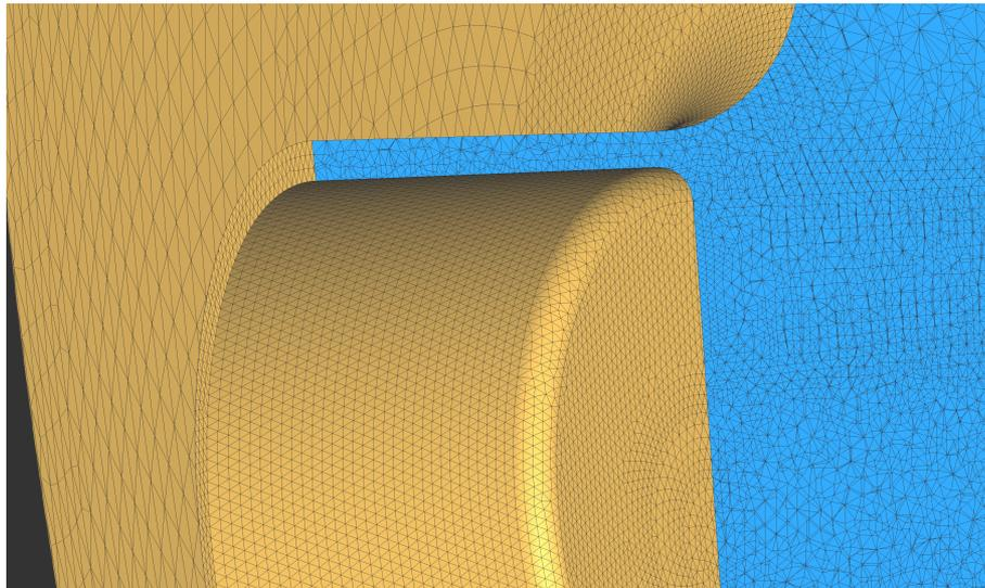
Cut-view of unstructured mesh near cathode
