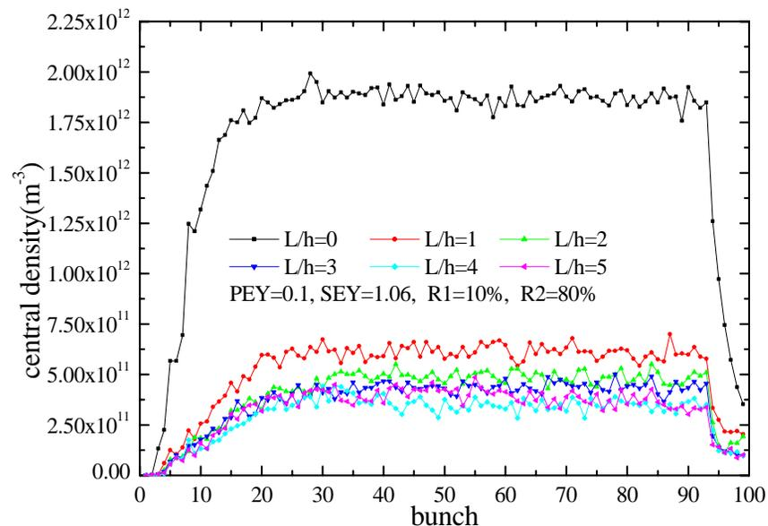
With the antechamber, the central density can be reduced about 5 times.
