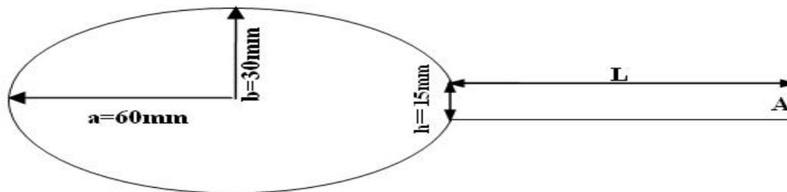
chamber structure in the simulation
