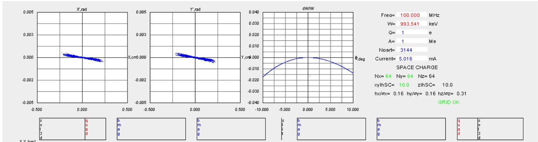
Manually optimized case :  $\epsilon(x, 80\%) = 0.090 \mu\text{m}$ ,  $\epsilon(y, 80\%) = 0.092 \mu\text{m}$
