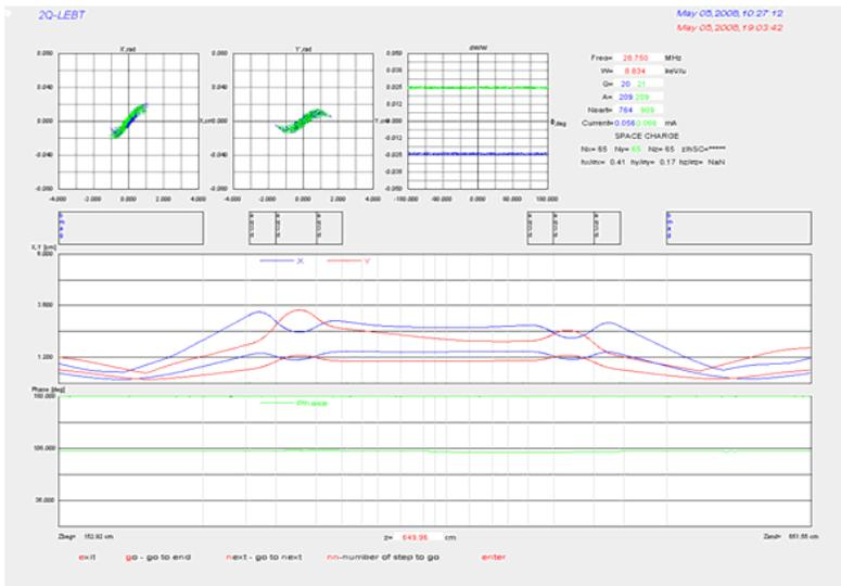
Measured beam profiles at the end of LEBT: left: horizontal, right: vertical.
