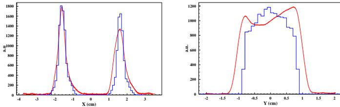
TRACK fit to find the quads setting to recombine the two charge state Bi-209 beams at the end of the LEBT.
