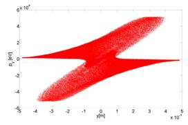
Figure 3: Electron distribution in the transversal (y) phase space after the passage of the ILC bunch.
