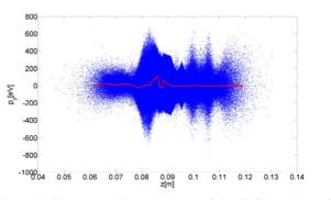
Figure 8: Transversal impulse  $(p_y)$  of the ILC bunch particles from Figure 7 after the passage through the e-cloud.
