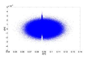
Figure 7: Profile of the ILC bunch with an offset slab in the middle part of the bunch.
