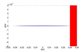
Figure 1: Longitudinal profile of the ILC bunch and the e-cloud, before the bunch enters in the cloud.
