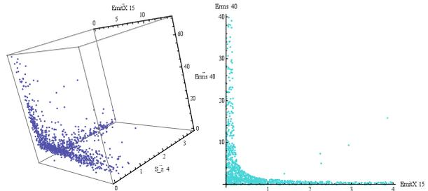
Figure 6: Left: Trade-off among solutions attempting to satisfy 3 parameters at the same time:  $\epsilon_N^X = 15$  mm-mrad,  $\sigma_Z = 4$  mm &  $\sigma_E = 40$  keV. Right: Solutions attempting to satisfy 2 parameters:  $\epsilon_N^X = 15$  mm-mrad &  $\sigma_E = 40$  keV, as well as additional constraints.
