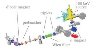
Figure 2: Schematic computational model of the compact injector design for the new polarized electron source at the S-DALINAC.
